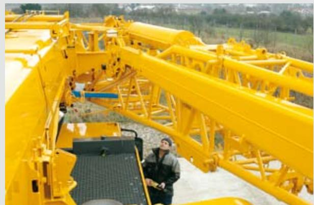
Hydraulic assembly assistance for attaching the folding jib
